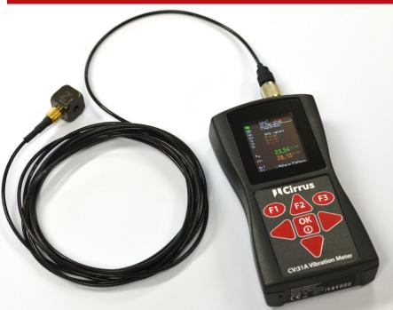
The CV:31A Revo<sup>™</sup> Vibration Meter provides a simple and convenient way to measure, analyse and assess vibration data in accordance with standards such as ISO 5349 and European Directive 2002/44/EC.
