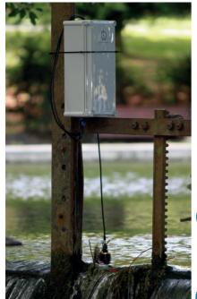
The AP-7000 has various output options: Aquaread standard output, SDI-12 and Modbus RS-485. Using these outputs the sonde can be connected to any number of telemetry or data logging devices.
